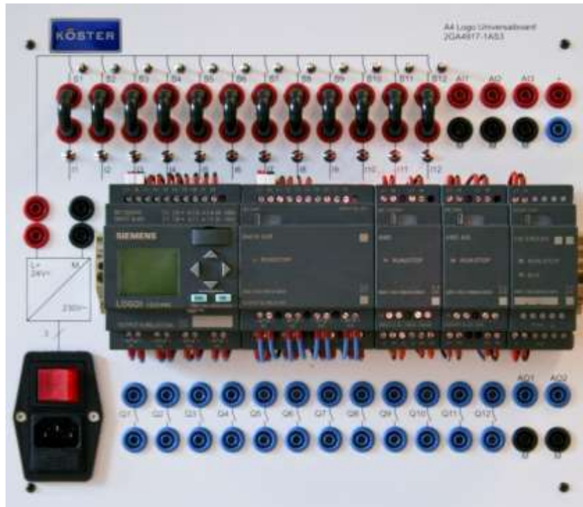
Fig.7 PLC Trainer by KOESTER (Encon, 2017)
