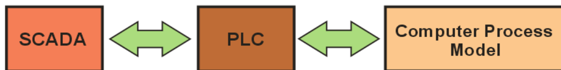
Fig.10 The physical control device connected with the computer model and process visualisation
