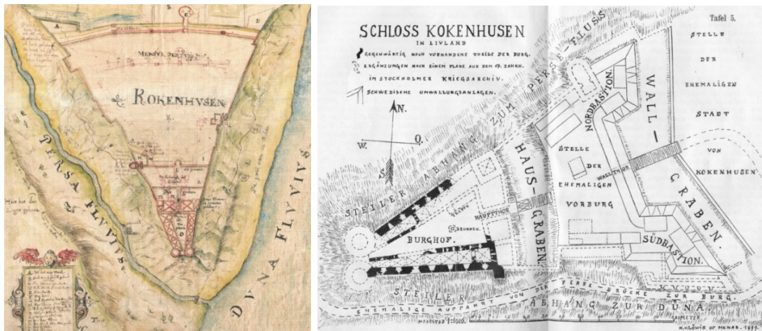
Figure 3 Fecit Georgius Schwengell. Plan of Kokenhusen Stronghold, castle-front and town: C – City Gate, E – town, F – church, H – tower, L – placement of the old wall, M – tall tower, N – bridge over the ditch, O – castle, P – towers, Q – Water Gate. Around 1630 (Stockholm, Kungl. Krigsarkivet)
