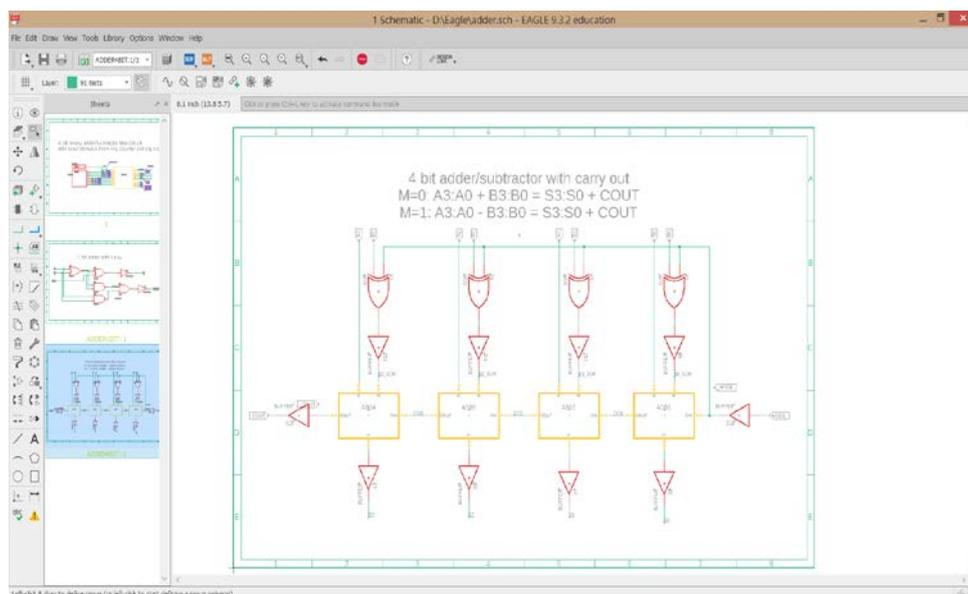
Figure 4 Four-bit adder circuit in Autodesk Eagle (Trajdos, 2020)
