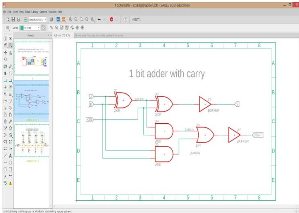
Figure 3 Single-bit adder circuit in Autodesk Eagle (Trajdos, 2020)
