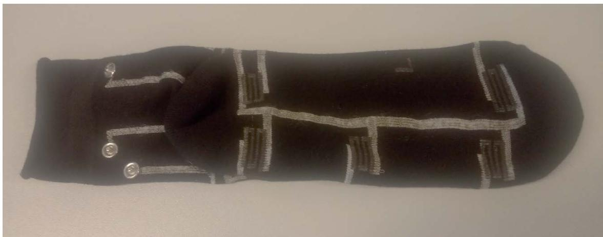
*Figure 1 Smart Socks system with 5 textile sensors*
