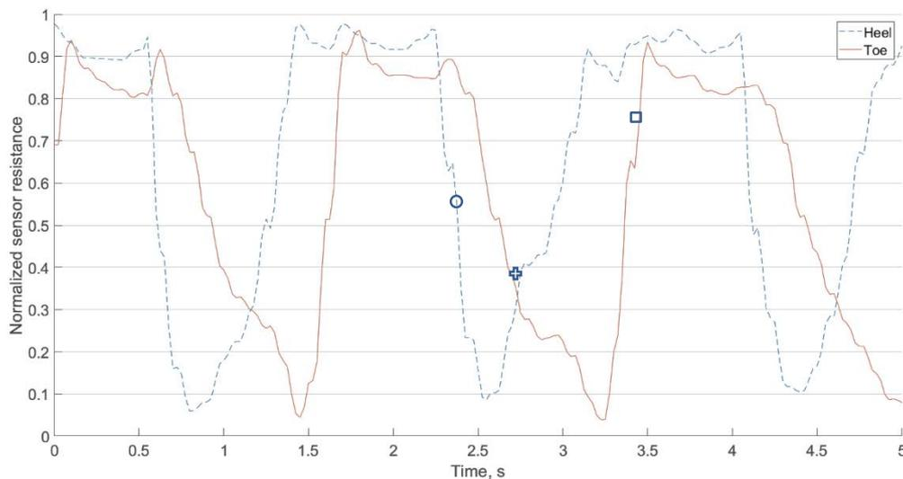
*Figure 4 Sensor signal example, heel touch (circle), flat foot (cross) and toe raise (square) detection moments are shown*
