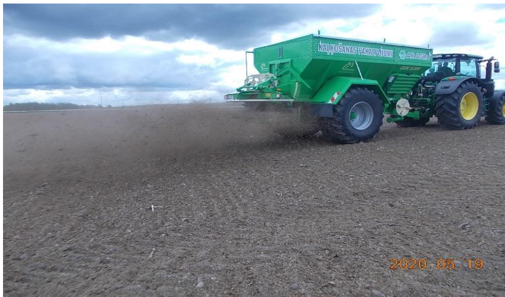
Spreading of digestate and wood ash mixture on the field.
