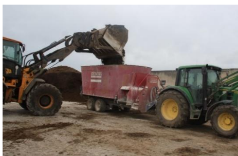
Preparation of raw materials for mixtures - digestate and wood ash, using front loader JCB 434S.
