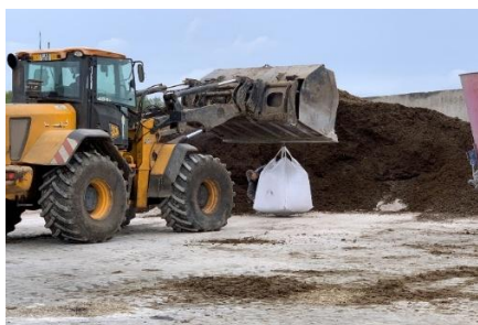
Preparation of raw materials for mixtures - digestate and wood ash, using front loader JCB 434S.
