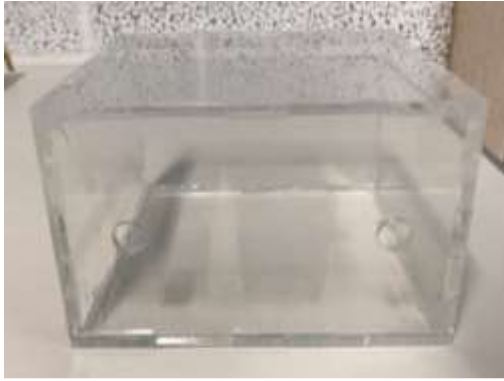
Image 1: Acrylic Box (150mm*100mm*150mm)
