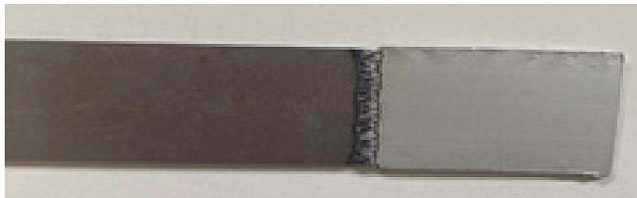
Fig.2. Sample of aluminum and iron welding
