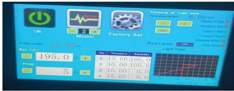
Fig.3. Fibre laser control panel
