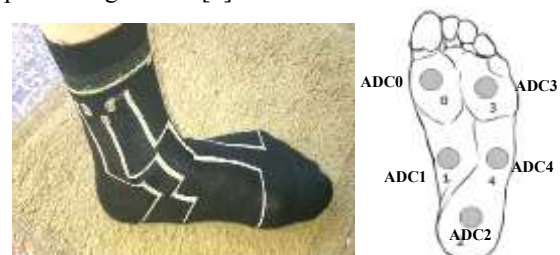
Fig. 1. Allocation of left foot sensors of Daid® Pressure Sock System.
