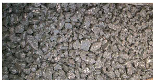
Fig. 1. Type of coarse-pored concrete
