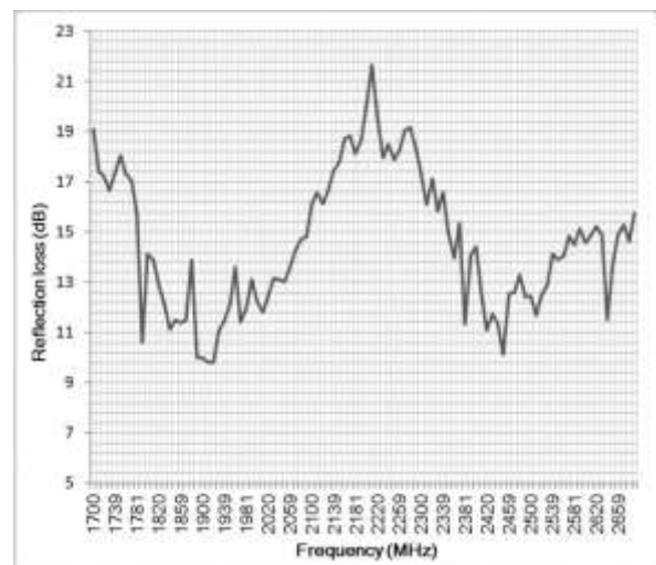
Fig. 8. Averaged reflection loss across all fresh snow thicknesses as a function of frequency.
