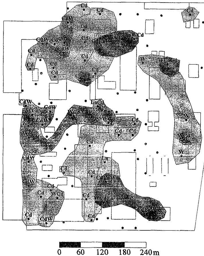
Fig. 4. Subdivision of "Ekranas" plant in Panevėžys into zones according to dangerous point summary pollution codes Notes: 1. The main association related with special glass (Sb, Pb, As), kinescopes (Li, Sr) and luminophores (Ba) production exceeds the allowable level on the whole territory of the plant. The codes of zones show the relative importance of additional pollution
