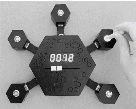
Fig. 2. Participant performs a task by pressing the small 0.5 cm buttons on the SnipTouch device prototype with a dowel.
