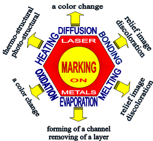
Fig. 2. Physical processes in laser marking on metals
