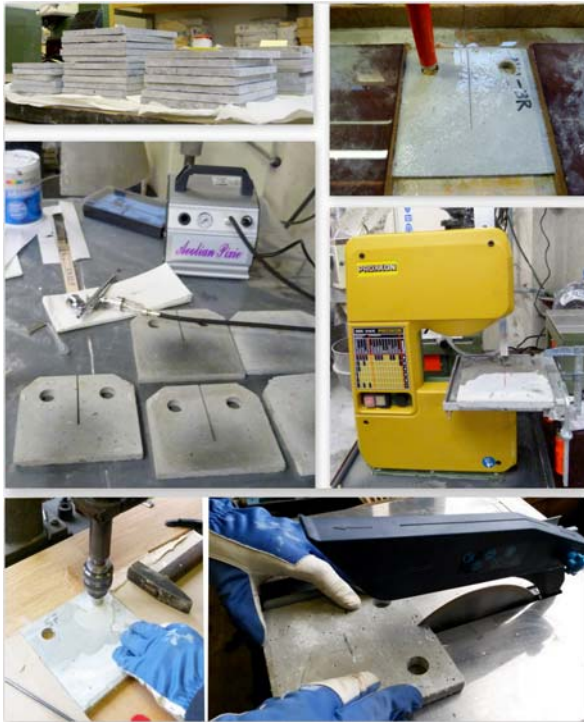
Fig. 2. Preparation of Compact Tension specimens
