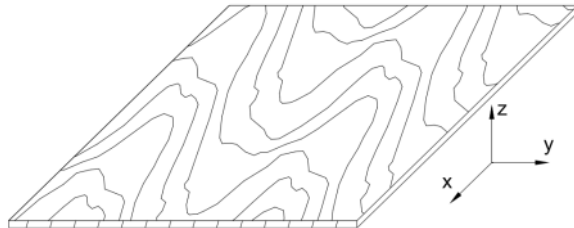
Fig. 4. Three principal axes of wood with respect to grain direction and growth rings. (x – longitudinal; y – tangential; z – radial) [13]
