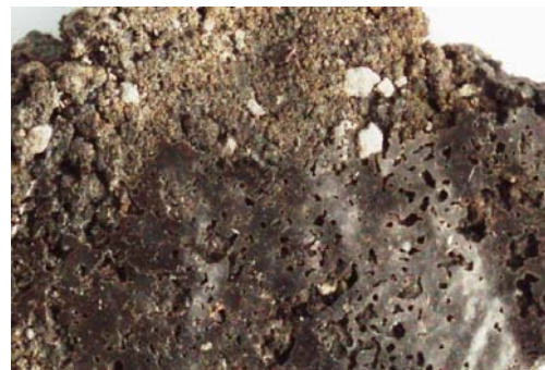
Fig. 4. Composite from mixture „Clay + PET”. PET content 30% (mass)
