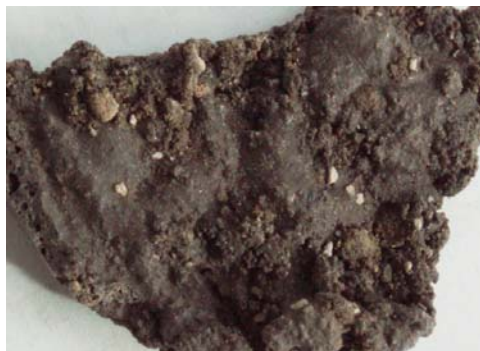
Fig . 6. Composite from mixture „ Ash+ PET"(volume of ash 50%)
