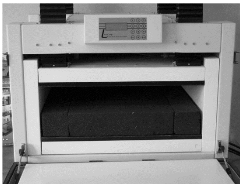
Fig. 3. Thermal conductivity measuring equipment FOX600 in RTU Faculty of Civil Engineering
