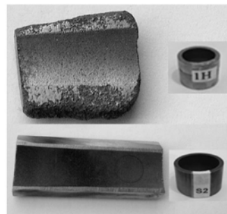
Fig.1. Fragments and view of powder parts after compacting (H1) and following sintering (S2): outer diameter 25 (45) mm, inner diameter 11 (29) mm, length 22 (31) mm correspondingly.
