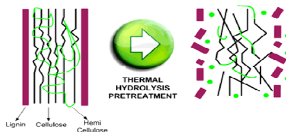
Fig. 1. Wood cell changes after SE processing [5].
