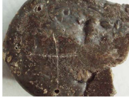
Fig 7. Composite from mixture „ Ash+ PET"(volume of ash 22% )
