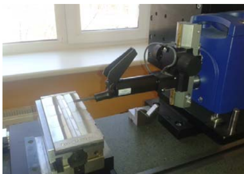
Fig.2. Measurement device Taylor Hobson Talysurf Intra 50
