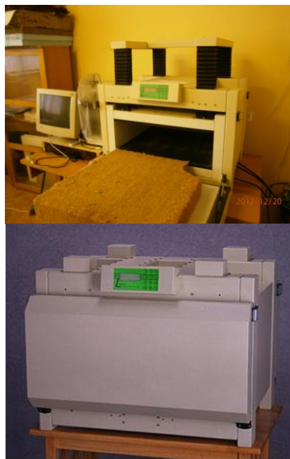
Figure 3. LaserComp FOX600 in the testing laboratory of building materials of the Riga Technical University.
