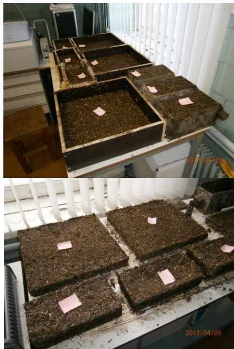
Figure 1. The drying process of the lightweight concrete of the new building material from sapropel and hemp shives
