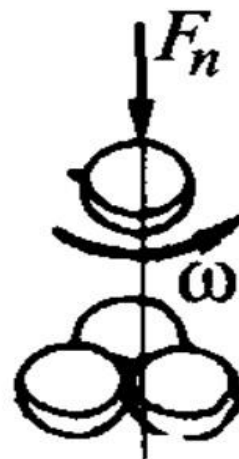
Fig.2. Four-ball test subassemblies principal block diagram
