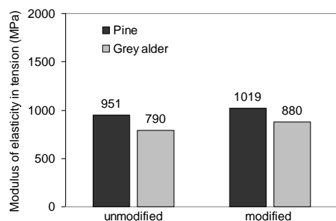
Fig. 3. Modulus of elasticity of polymer composites filled with initial and modified wood bark
