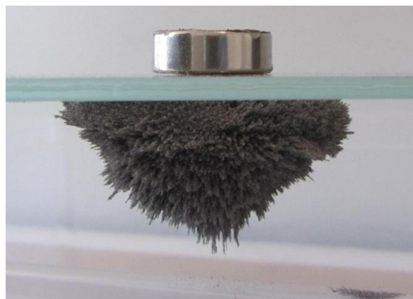
Fig. 1. CS retaining by a magnet
