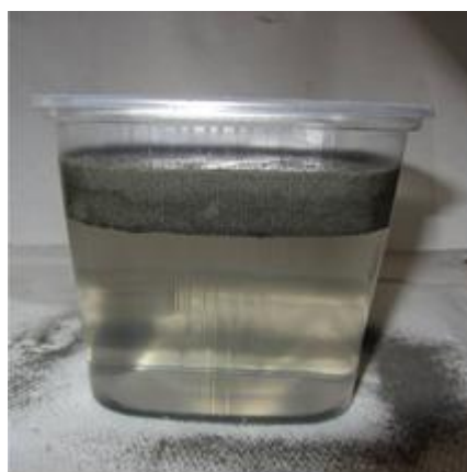
Fig. 2. CS retaining on a water surface
