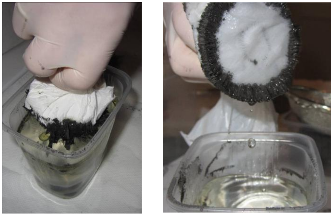
Fig. 11. Model of an iron powder particle MH 80.23, moistened by water (inside pores) and oil (a double contour over entire external surface of particles)
