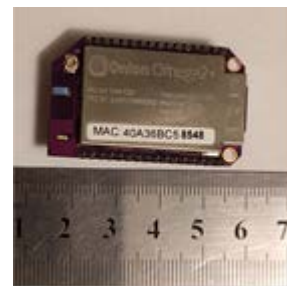
Fig. 5. Onion Omega2+ Linux Compute Module
