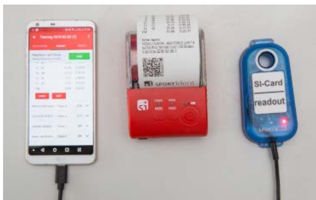
Fig. 5. Integrated SPORTident RFID data readout, event management and results printout system
