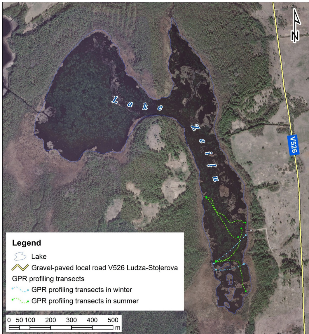
Fig. 1. GPR measurement lines lake Zeiļu in March 16, 2018 and June 8, 2018
