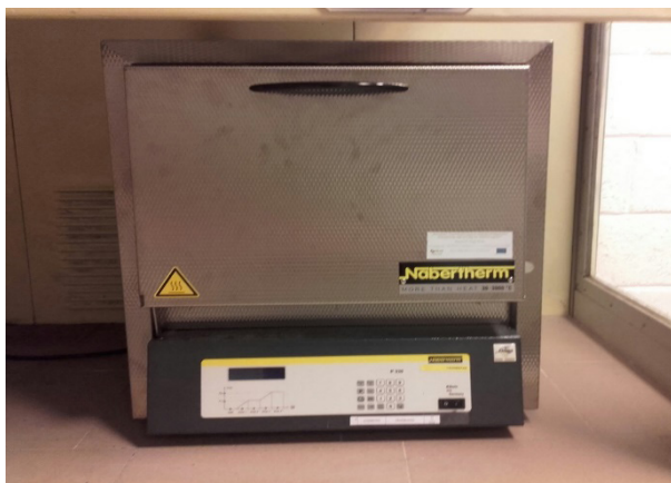
Fig. 2. The furnace used to determine the ash content After combustion in the furnace at the temperature
