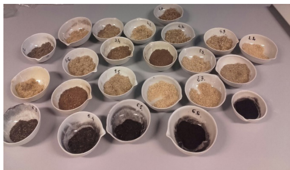
Fig. 1. Samples analysed to determine the ash content For combustion of samples the furnace “Nabertherm” was used (Fig. 2).
