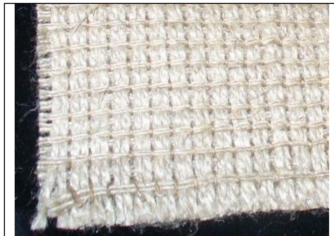
Fig.3. Sample of the woven reinforcement structure. Flax multi-layer overlaid weave 2/2
