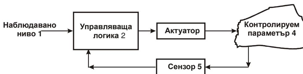
**Fig.1. Generally accepted model of micro-system**
