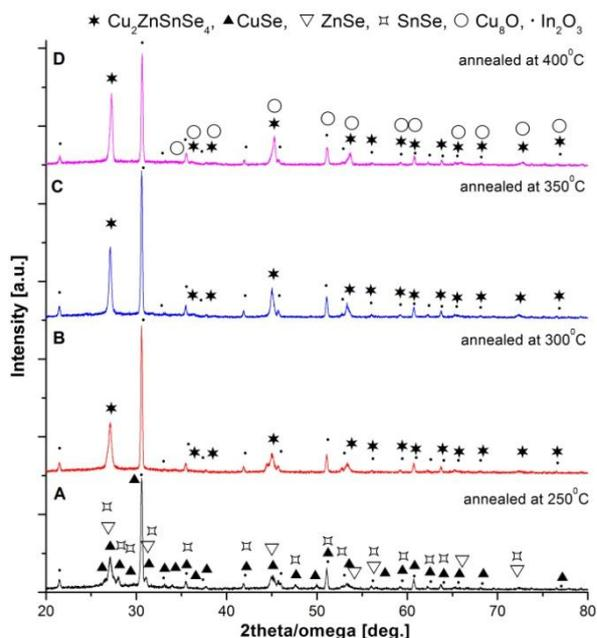
Fig. 3. X-ray diffractometry data of  $Cu_2ZnSnSe_4$  films annealed at: a)  $250^{\circ}C$ ; b)  $300^{\circ}C$ ; c)  $350^{\circ}C$ ; d)  $400^{\circ}C$ .
