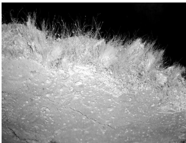
Figure 3. Short AR glass fibers homogeneously distributed in the concrete shell
