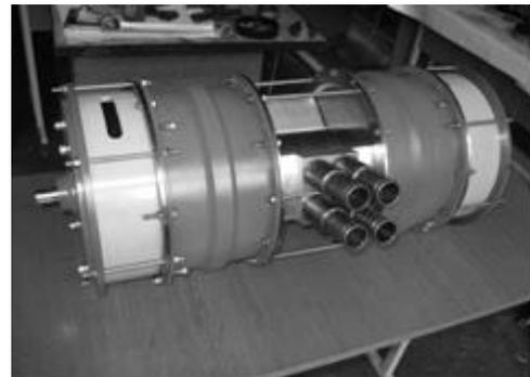
Fig. 1. Rotary-vane external combustion engine.
