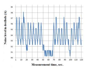
Pic. 2 Noise level at the workplace during wood processing
