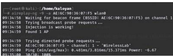
Fig. 5 Injection of packets in experimental Wi-Fi network.
