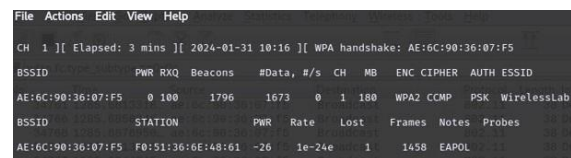
Fig. 6 View of terminal with use of airodump-ng
