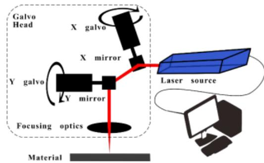
Figure 1: Schematic view of Rofin powerline laser system
