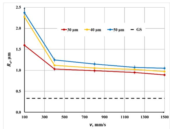
Figure 10b: Graphics of the dependence of the roughness on the speed from 100 mm/s to 1500 mm/s for three raster steps for one-time marking
