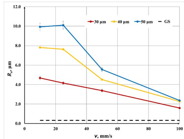
Figure 10a: Graphics of the dependence of the roughness on the speed from 10 mm/s to 100 mm/s for three raster steps for one-time marking
