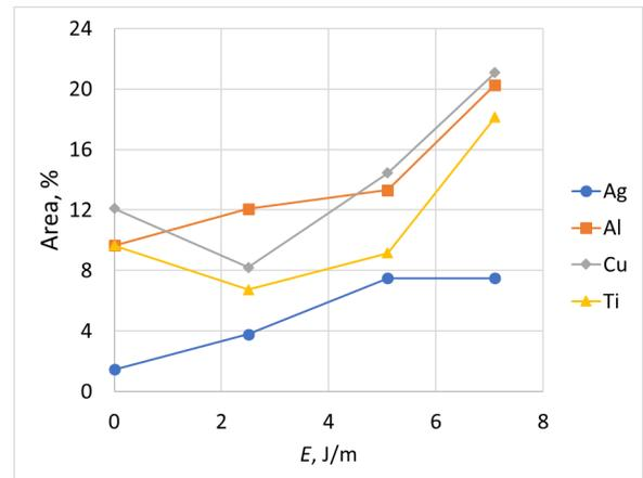
Fig.6. Peeled off adhesion test results of deposited metals on Fabric C dependent on laser linear energy density.
