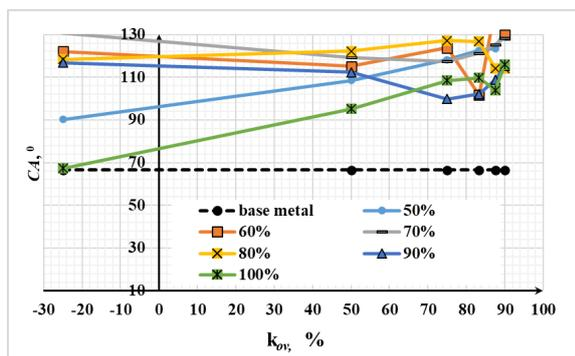
Fig. 13. Contact angle dependence on pulse overlap and power.
