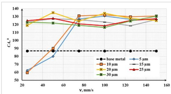
Fig. 8. Contact angle dependence on the scanning speed.
