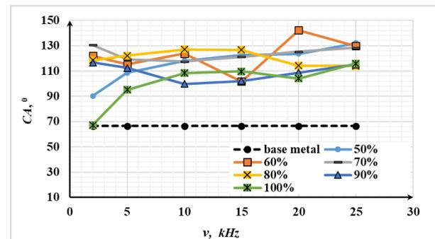
Fig. 11. Contact angle dependence on the frequency.
