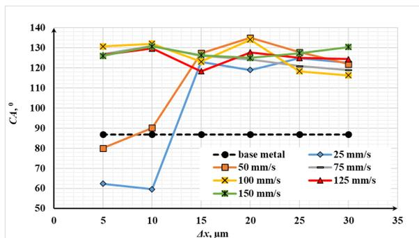
Fig. 9. Contact angle dependence on the raster step.
