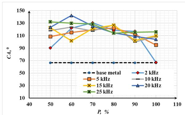
Fig. 12. Contact angle dependence on the average power.
