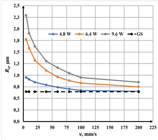
Fig 8. Dependence of the roughness  $R_a$  on the speed  $v$  during laser marking of a sample of stainless steel for powers  $P$ : blue color - 4.8 W, orange color - 6.4 W, gray color - 9.6 W and GS – ground (untreated) surface.
