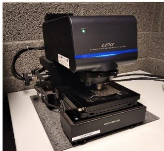
Fig. 1. Lext 3D measuring laser microscope OLS5000
