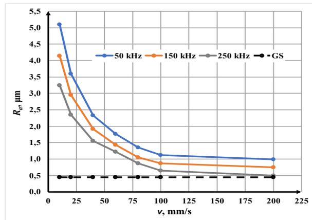
Fig 12. Dependence of the roughness  $R_a$  on the speed  $v$  during laser marking of a sample of stainless steel for frequencies  $\nu$ : blue color – 50 kHz, orange color – 150 kHz, gray color – 250 kHz and GS – ground (untreated) surface.
