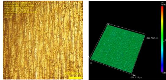
Fig 11. Marked square with smallest roughness  $R_a$  for the second sample
