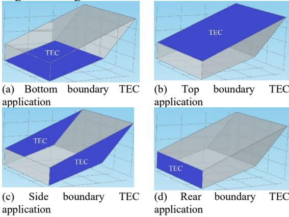
Fig. 2. TEC placements on the glove compartment
