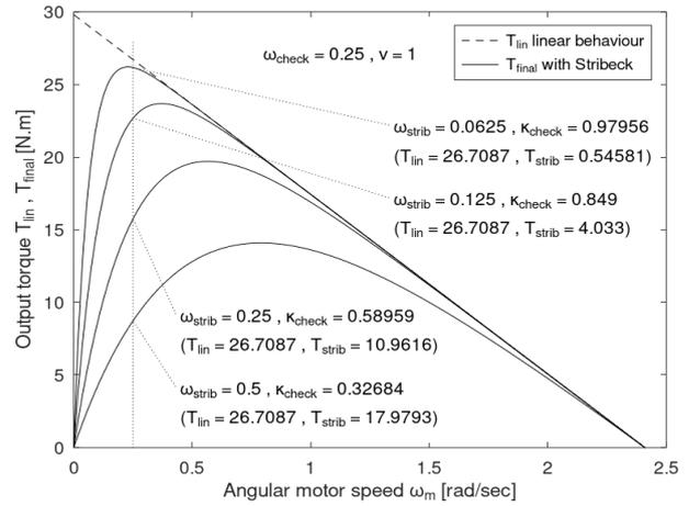
Fig. 2. Plot of Stribeck caused losses at fixed sharpness factor  $\nu$  and different Stribeck critical speeds  $\omega_{\text{strib}}$ .
