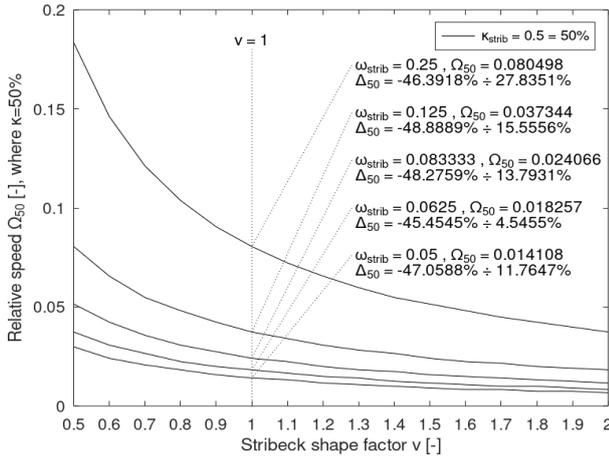
Fig. 4. Plot of speeds  $\omega_{50}$  when Stribeck losses are  $\kappa_{50} = 50\%$ , but given as relative speed  $\Omega_{50} = \omega_{50}/\omega_{noload}$  at different Stribeck critical speeds  $\omega_{strib}$  and different sharpness factors  $\nu$ .
