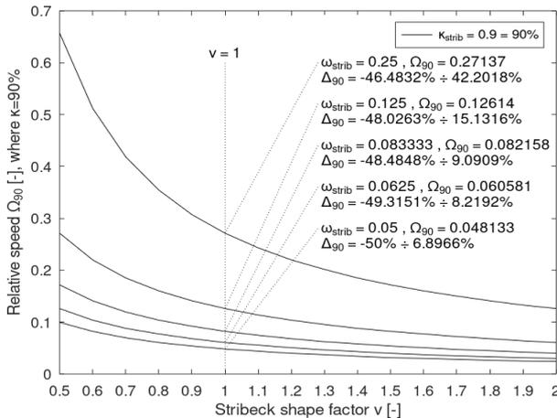
Fig. 5. Plot of Stribeck losses  $\kappa_{90} = 90\%$  appearance at some speed  $\omega_{90}$ , but given as relative speed  $\Omega_{90} = \omega_{90}/\omega_{noload}$  at different Stribeck critical speeds  $\omega_{strib}$  and different sharpness factors  $\nu$ .
