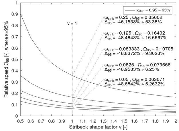
Fig. 6. Plot of Stribeck losses  $\kappa_{95} = 0,95\%$  appearance at some speed  $\omega_{95}$ , but given as relative speed  $\Omega_{95} = \omega_{95}/\omega_{noload}$  at different Stribeck critical speeds  $\omega_{strib}$  and different sharpness factors  $\nu$ .
