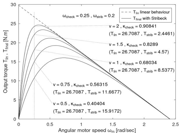
Fig. 3. Plot of Stribeck caused losses at fixed Stribeck critical speed  $\omega_{\text{strib}}$  and different sharpness factors  $\nu$ .
