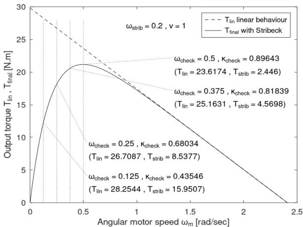
Fig. 1. Plot of Stribeck caused losses at fixed Stribeck critical speed  $\omega_{\text{strib}}$  and fixed sharpness factor  $\nu$ .
