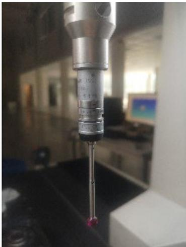
Fig. 2. TP20 sensor with D6 probe.
