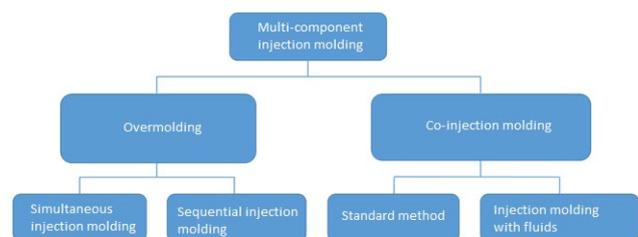
Fig. 1 Classification of multicomponent injection molding processes
