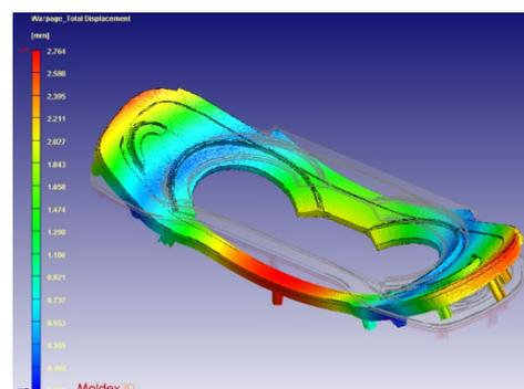
Fig. 13 Total displacement
