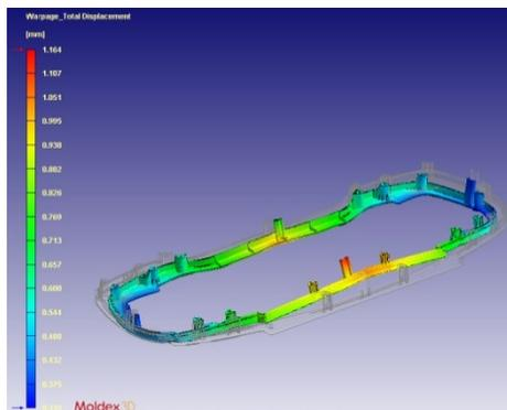
Fig. 8 Total Displacement
