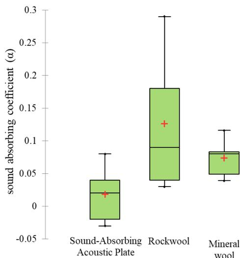
Fig. 8. Sound absorption coefficients at low frequencies (100-250 Hz)
