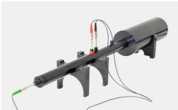
Fig.5. Sound Absorption impedance tube [10]
