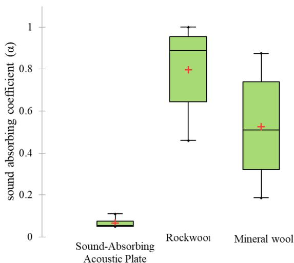
Fig. 9. Sound absorption coefficients at medium frequencies (315 - 1000 Hz)
