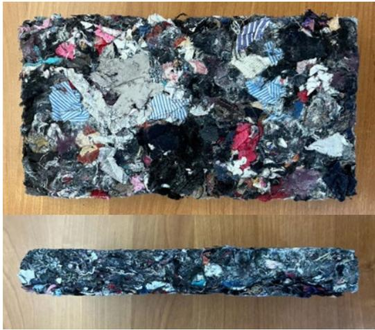
Fig. 4. Sound-Absorbing Acoustic Plate
