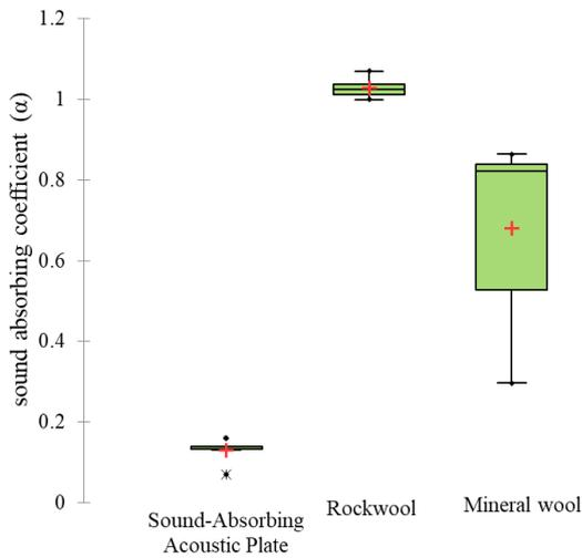
Fig. 10. Sound absorption coefficients at high frequencies (1250 - 4000 Hz)
