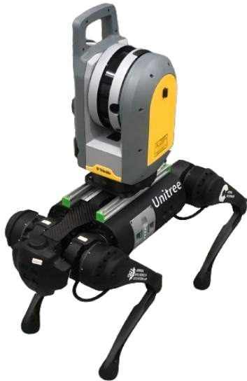
Fig. 5. Trimble X7 mounted on the back of Unitree Go 1 Edu using the constructed fastening device.
