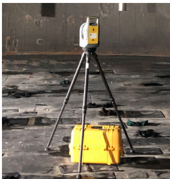
Fig. 2. Trimble X7 3D laser scanning system.
