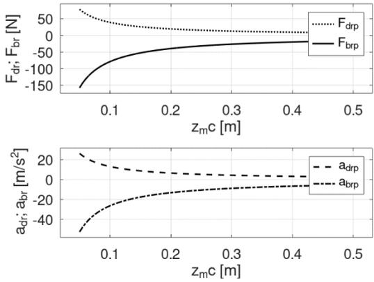
Fig. 12. Permissible forces and accelerations according to  $z_{mc}$  value and  $l = 0.4$ , ( $l_r = \frac{1}{3}l$ ;  $l_f = l - l_r$ ), i.e.  $K_{base} \neq const$ .
