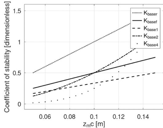
Fig. 3. Coefficients of stability according to  $z_{mc}$  value and  $l = 0.3$ , ( $l_r = \frac{1}{3}l$ ;  $l_f = l - l_r$ ).
