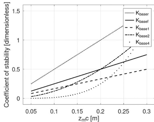
Fig. 4. Coefficients of stability according to  $z_{mc}$  value and  $l = 0.6$ , ( $l_r = \frac{1}{3}l$ ;  $l_f = l - l_r$ ).
