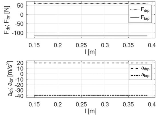
Fig. 14. Permissible forces and accelerations according to  $l$  value when  $l_r = \frac{1}{3}l$ ;  $l_f = l - l_r$ ;  $z_{mc} = \frac{1}{6}l$ , i.e.  $K_{base} = const$  (see Fig. 13). But here  $F = const$  only when  $m = const$  “(10), (11)”.
