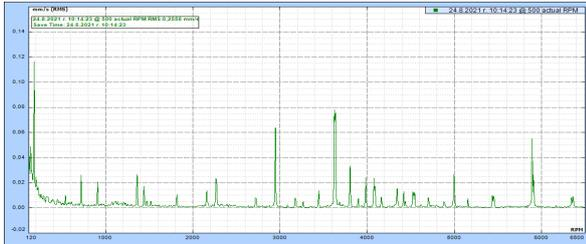
Figure 2 Spectrum of oscillations of Stern tube bearing right shaft line.
