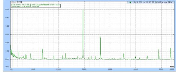
Figure 4 Spectrum of oscillations of Stern tube bearing right shaft line.
