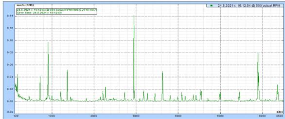
Figure 3 Spectrum of oscillations of Stern tube bearing right shaft line.
