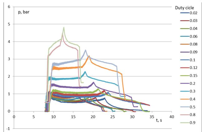
Fig. 5. Variation of pressure in the left chamber of the pneumatic cylinder with double out rod at different values of the duty cycle 20 Hz.
