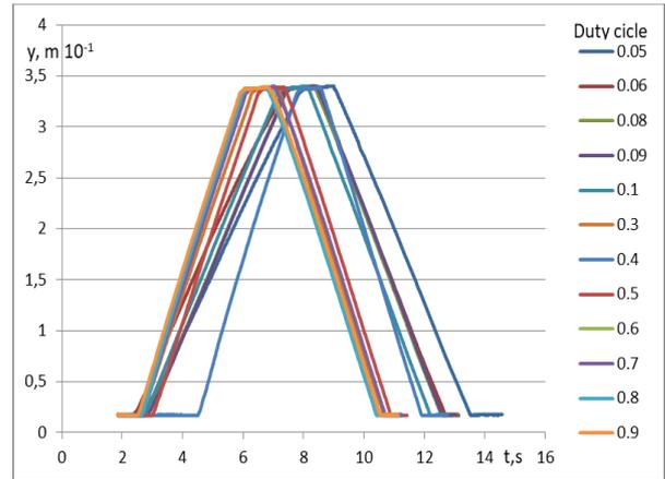
Fig. 15. Displacement of the piston of the pneumatic pistonless cylinder at different values of the duty cycle 70 Hz.
