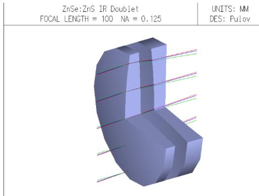
Fig. 2. Optical system layout of the IR doublet
