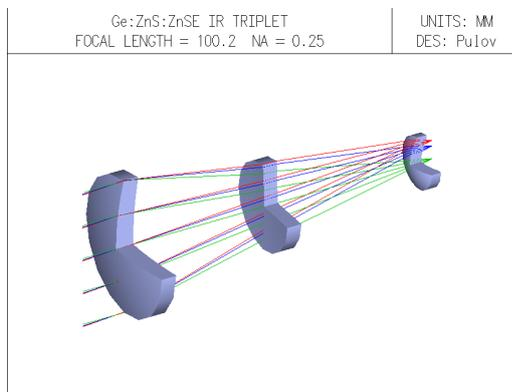
Fig. 3. Optical system layout of the IR triplet
