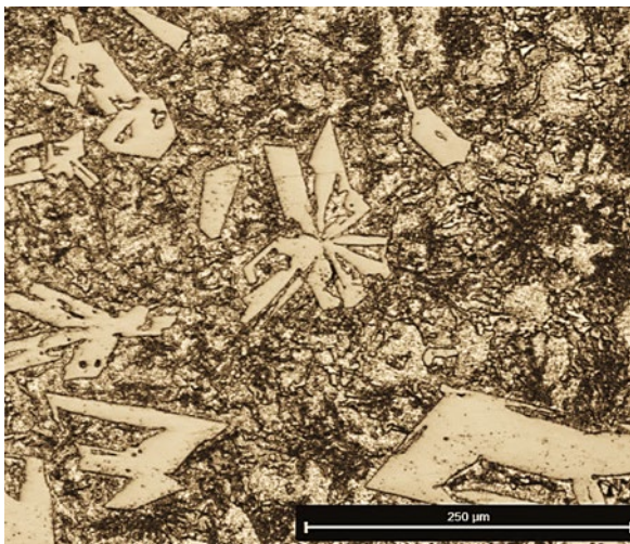
Fig. 2. Microstructure of AlSi21Cu5Cr alloy (pure metals)
