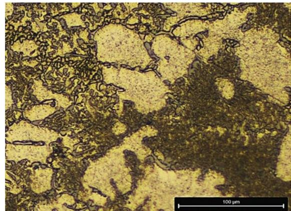
Fig. 1. Microstructure of AlSi12Cu5Mn alloy without heat treatment
