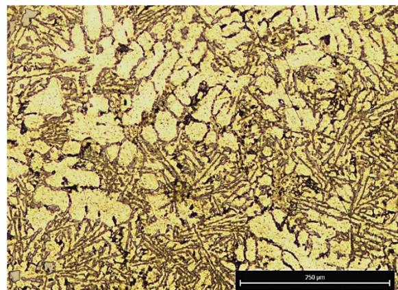
Fig. 2. Microstructure of AlSi12Cu5MgCr alloy without heat treatment
