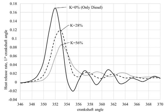
Fig. 5. Heat release rate of D3900 at 45% load and 1400 min<sup>-1</sup>.
