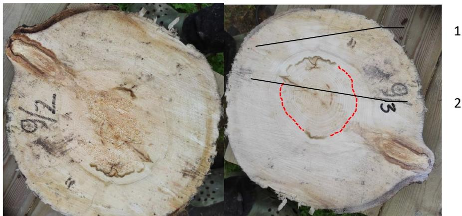
Fig. 8. The identification of the heartwood coloured timber, where: 1- demarcation line; 2- the heartwood coloured timber
