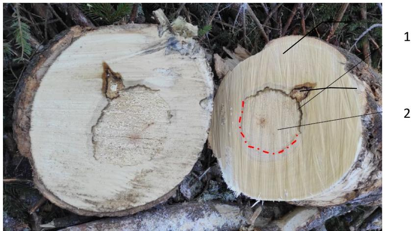
Fig. 7. The identification of the heartwood hard rot, where: 1- demarcation line; 2- the heartwood hard rot stage timber.
