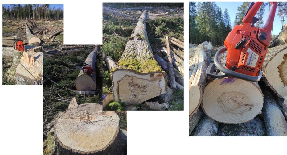
Fig. 2. Preparation of selected aspen stems quality characterized wood pieces for fungal identification.
