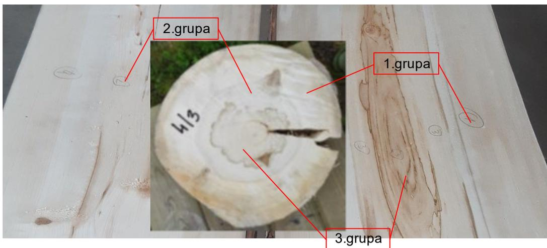
Fig. 5. Selecting of the testing samples according to the quality, where 1 grupa- sound timber, 2 grupa- heartwood coloured timber, 3 grupa- heartwood hard rot stage timber.
