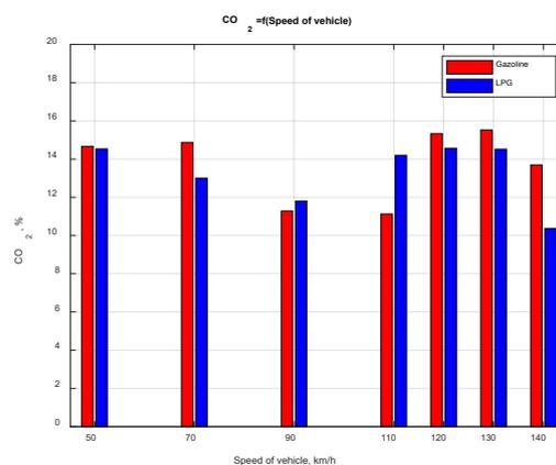
Fig. 8. Experimental study of the content of CO<sub>2</sub>, [%] in the exhaust gases of a car Honda Civic Aerodeck 1.5 iLS.
