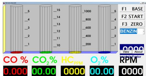
Fig. 4. Full screen mode of the DEK DG-04IR gas analyzer software.
