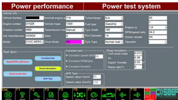
Fig. 2. Window with the technical data of the tested car [8].
