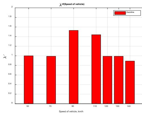
Fig. 10. Experimental study of the content of  $\lambda$  in the exhaust gases of a car Honda Civic Aerodeck 1.5 iLS.
