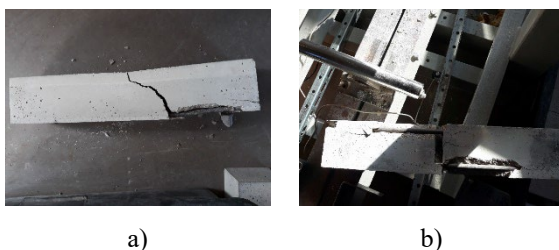
Fig. 8. Destruction mode of beam with steel reinforcement (a) and titanium reinforcement (b).
