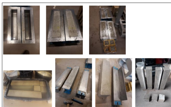
Fig. 5. The process of production of reinforced concrete and titanium concrete beams.
