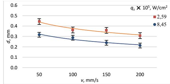
Fig. 11. Dependence of the line width  $d$  on scan speed  $v$  at two different power density  $q_s$  for aspen thermowood sample heat-treated at 225°C.
