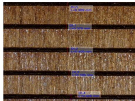
Fig. 7. Line width measurement (magnification x32) - aspen thermowood sample heat-treated at 214°C.
