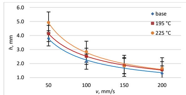
Fig. 15. Dependence of the line depth  $h$  on scan speed  $v$  at power density  $q_s = 8.45 \cdot 10^5$  W/cm<sup>2</sup>.
