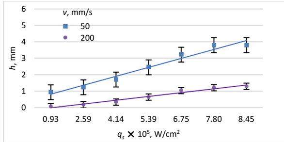
Fig. 12. Dependence of the line depth  $h$  on power density  $q_s$  at two different scan speed  $v$  for the sample of natural aspen.
