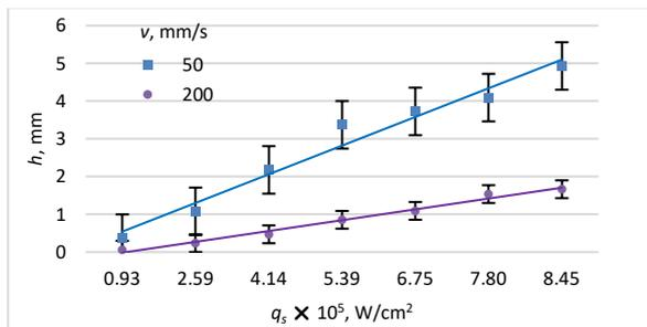
Fig. 13. Dependence of the line depth  $h$  on power density  $q_s$  at two different scan speed  $v$  for aspen thermowood sample heat-treated at 225°C.
