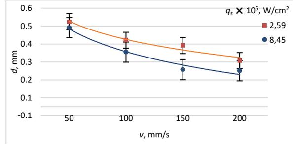
Fig. 10. Dependence of the line width  $d$  on scan speed  $v$  at two different power density  $q_s$  for aspen thermowood sample heat-treated at 180°C.
