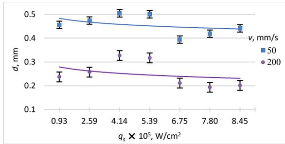
Fig. 8. Dependence of the line width  $d$  on the power density  $q_s$  at two different scan speed  $v$  for aspen thermowood sample heat-treated at 180°C.
