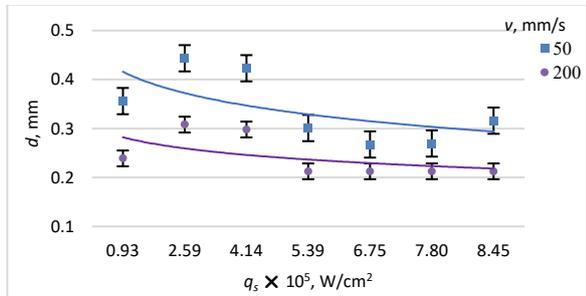
Fig. 9. Dependence of the line width  $d$  on the power density  $q_s$  at two different scan speed  $v$  for aspen thermowood sample heat-treated at 225°C.
