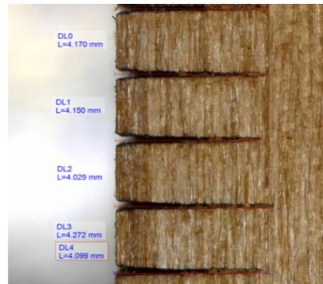
Fig. 6. Measurement of engraving depth on an aspen thermowood sample that was heat-treated at 195°C. (magnification x32).
