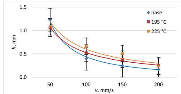
Fig. 14. Dependence of the line depth  $h$  on scan speed  $v$  at power density  $q_s = 2.59 \cdot 10^5$  W/cm<sup>2</sup>.
