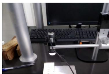
Fig. 3. Dino-Lite Edge AM7115MZT digital microscope.
