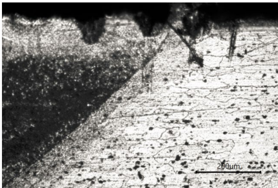
Fig. 4. Grain size of the base and stirred metal (regime 1.1).
