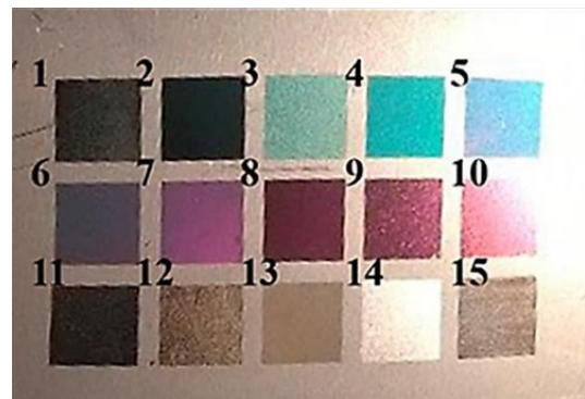
Figure 16. Color palette after 24 hours of environmental exposure in the test chamber at -40 °C and 90% humidity.
