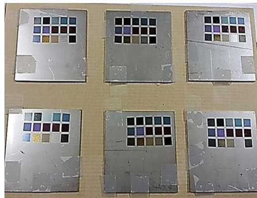
Figure 13. Six identical color palettes produced with the same laser processing parameters.
