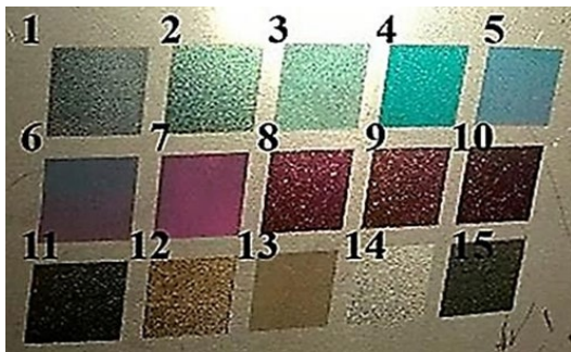
Figure 18. Color palette after 24 hours of environmental exposure in the test chamber at 40 °C and 70% humidity.
