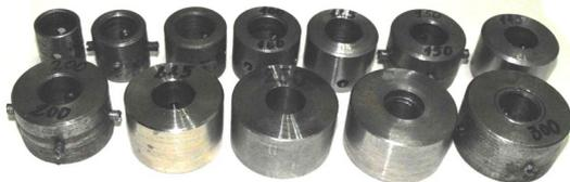
Fig. 8. Masses that were mounted on barrel edge with values 0,025; 0,05; 0,075; 0,100; 0,125; 0,150; 0,175; 0,200; 0,225; 0,250; 0,275; 0,300 kg.
