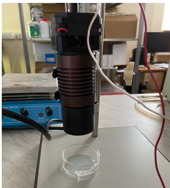
Fig. 2. Experimental set-up for irradiation tests.
