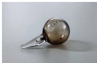
Fig. 1. Typical design of the high-frequency light source.
