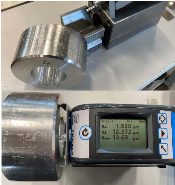
Fig.6 Scheme of the experimental installation for taking data on the roughness of the treated surface
