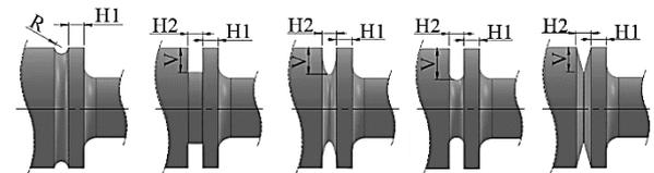
Fig. 4. Geometric parameters and shapes of the notches used in the simulation of the stepped specimen.
