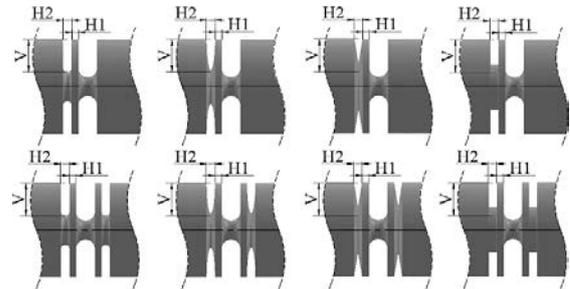
Fig. 2. Geometric shapes of the notches in the cylindrical specimen with a central U-notch.
