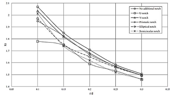
Fig. 5. Stress concentration coefficients for all studied cases, as a function of the geometric ratio  $r/d$ .
